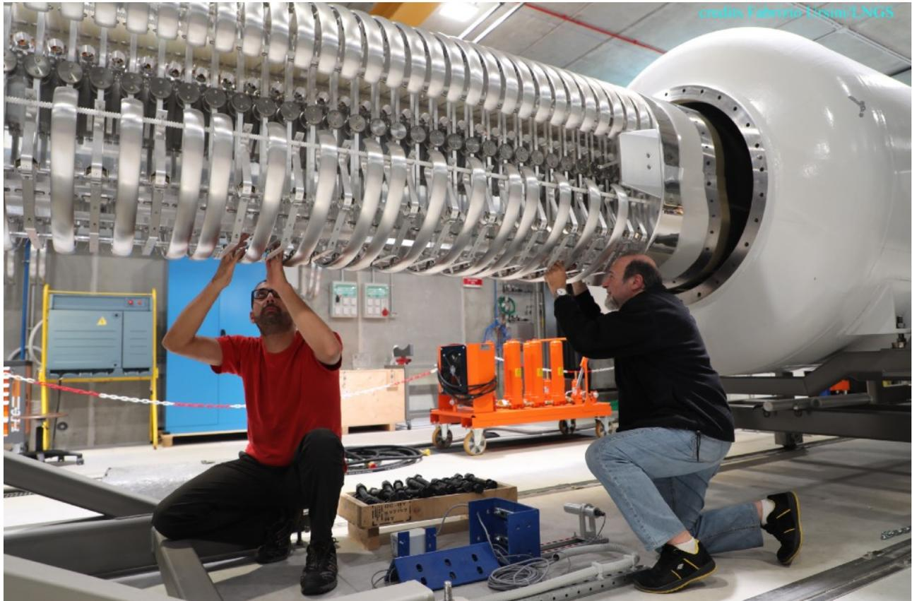
Figure 8. Maintenance on the 3.5 MV accelerator installed in the underground laboratories.
